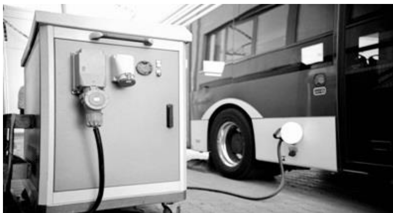
Rys. 3. Ładowanie elektrobusem metodą plug-in [17] Fig. 3. Charging of an electric bus by plug-in method [17]
